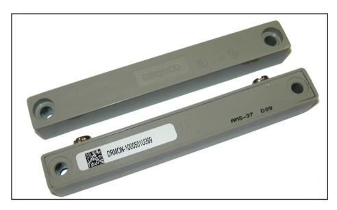
DRMON-1 is a magnetic contact switch that provides a signal to your Danfoss nvironment control system to ensure that the doors on refrigerated walk-in boxes are properly closed when not in use. The DRMON-1 is typically set to alarm in the closed position, indicating that a door has been left open.
