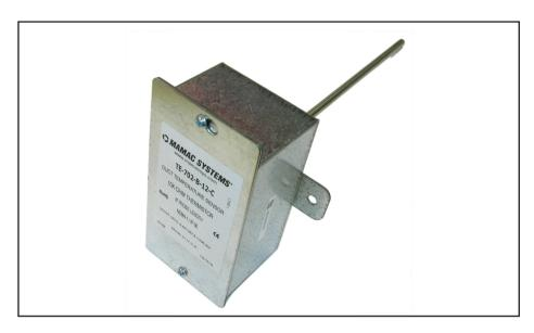
The 080Z2183 is a duct mounted temperature sensor that is used with the 080Z2180, 080Z281, or 080Z2182 thermostat. It is used to verify the operation and output efficiency of the heating and cooling stages. The 080Z2183 uses a thermistor sensor in a galvanized steel enclosure and is usually mounted in the supply or return ducts of an HVAC system.
