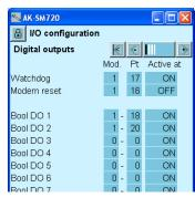
During I/O configuration, the position of the output must be defined.
