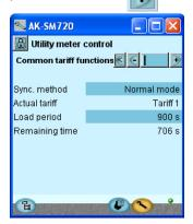
This function will require a signal from a pulse counter. Consumption can then be monitored in the screens displayed. Up to eight measurements can be set up.
