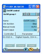
The groups that are set up via this control can collect signals from one On/Off function in any controller on the network.
