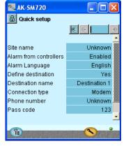
In this menu the necessary settings have been gathered so that a simple alarm routing can be established. All settings will be transferred to other respective displays.
