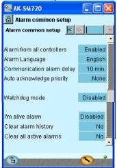
Set that alarms should be received from all the connected controllers.
