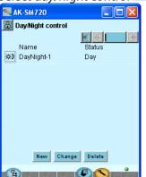
Groups established via this operation receive the day/night signal at the same time. Activation of the signal either takes place from a schedule and/or from a switch.
