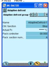
A group created via this control will use the "Adaptive defrost" function. The controllers in the group receive signals of the current condensation temperature from the condenser control.
