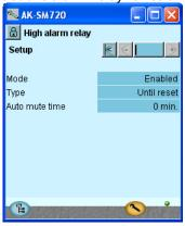
If the relay is to be activated by high priority alarms you must select the top line. Press the icon to proceed to the next page.
