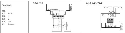
In general, the data communication is connected from controller to controller, so that L is connected to L, and H is connected to H. **The cable must be twisted in pairs and with screen.**
