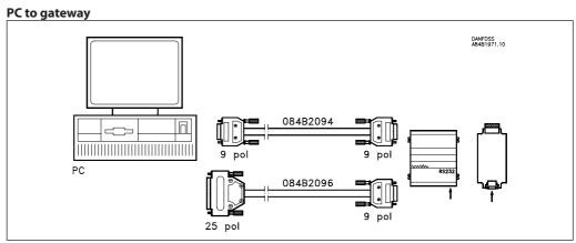
Check whether the PC has a 9-pole or a 25-pole plug for this connection. A 3 m cable with plugs fitted can be supplied. See Ordering. If the cable has to be longer than 3 m, mount it based on the following instructions:
