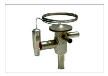
TUB/TUBE stainless steel thermostatic expansion valves are used for liquid injection into evaporators on both refrigeration and air conditioning systems using fluorinated refrigerants. TUB/TUBE valves are compact in design, light weight and have steel / copper bi-metal connections for fast soldering.TUB/TUBE have a fixed orifice and adjustable superheat.
