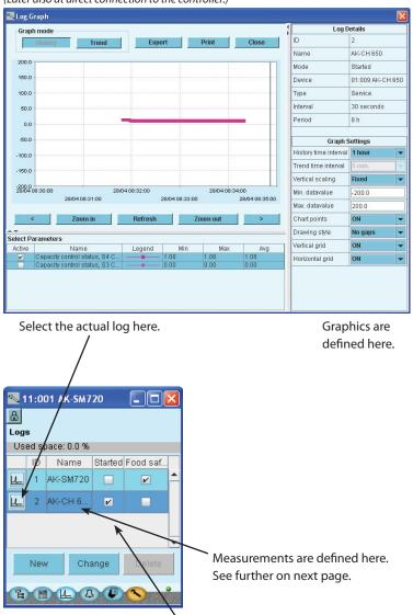
Data collection starts when the set-up is locked and the controller is started and start is activated.
