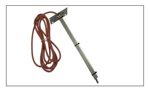
The ASTP2 air supply/duct sensor is a 084N2003 AKS21M sensor supported by a steel shaft that is used to verify the operation and output efficiency of stages of heating or cooling. It can also be used in conjunction with air control strategies employing temperature differential between supply and return air temperatures. The ASTP2 is typically mounted in the supply or return air ducts of an HVAC system
