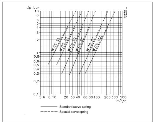
The capacity curves show the capacity (water quantity in m³/h) of the individual valve sizes as a function of pressure drop across the valve.
