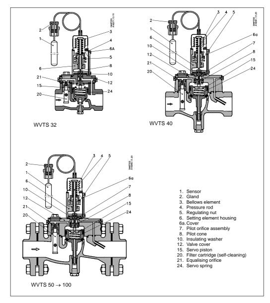
The valve body is made of cast iron with pressed-in bronze seat.
