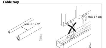
When the cable is ducted with other cables, there is a strong risk that electrical noise will be transferred. Keep away from live cables.
