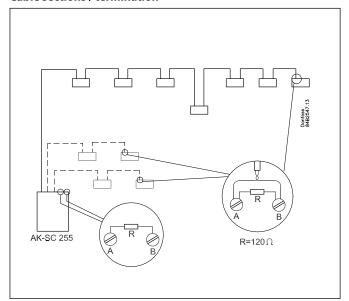
When all cables have been mounted on the different devices, the cable must be terminated.
