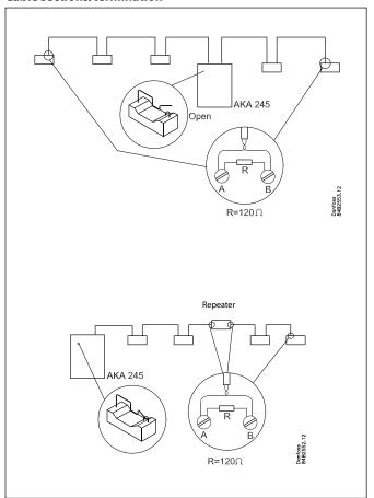
When all cables have been mounted on the different units, the cable must be terminated.
