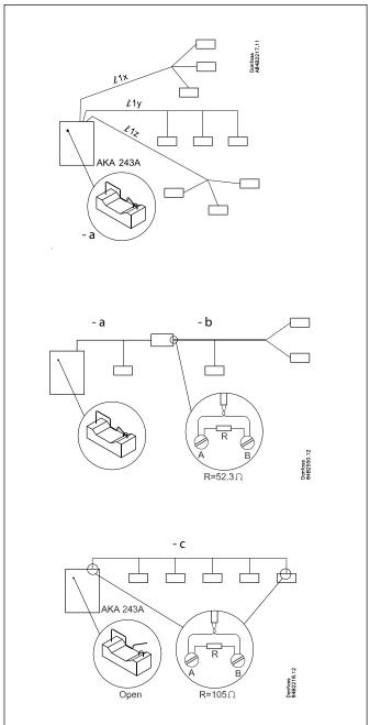
When all cables have been mounted on the different devices, the cable sections must be terminated. Short sections are only terminated at one end. Long sections, as shown on the bottom drawing, must be terminated at both ends.
