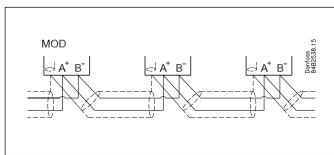
The wires are looped from device to device.
