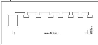
The cable is connected from controller to controller, and **no** branches are allowed on the cable.
