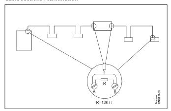
When all cables have been mounted on the different devices, the cable must be terminated.
