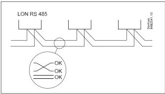
The two wires are looped from device to device. There are no polarisation requirements.
