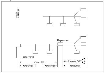
The wiring is optional, and branches are allowed on the cable.
