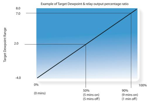
Relay output percentage (based on cycle time setting)
