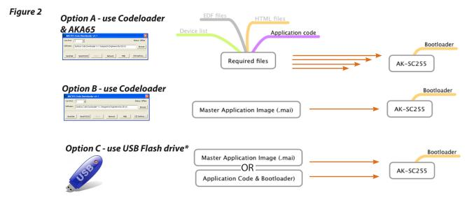
\*Loading via USB requires AK-SC255 V1.2 CPU card & above. Bootloader 6.1 must have already been installed.
