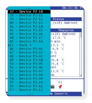
Whilst in the upper section of the Evap summary screen the use of the drop down box can be used to quickly access other controllers on the network. This feature is especially useful if there is a large network present.
