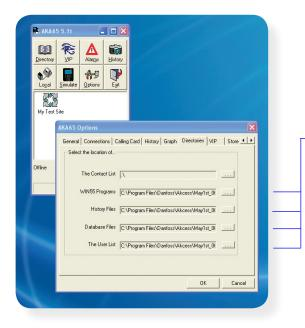
The WIN55 file is represented as a  $\stackrel{\text{def}}{=}$  icon and is the program that the AKA65 uses to run the AK-SC255 environment. Ensure that the AKA 65 directories points to the folder that holds this file. The 'E' version of the AK-SC255 is denoted by the file name 'VExx\_xxx.exe'
