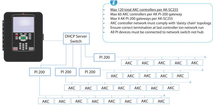
Assuming the PI-100 or 200 has been configured and the controller network is wired and addressed correctly, take the following steps to scan on the devices to the AK-SC255.
