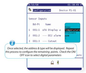
Once all parameters have been selected and (if) alarms limits are required, navigate to the **Alarm Configuration** screen (Main Menu/ Configuration/Alarms/). Select and enter the Miscellaneous icon and (dependent on sensor type) select the correct icon to display Miscellaneous sensor Alarms.
