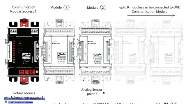
In the above example the AK-SC255 Board & Point address structure will be **01-2.7** The Communication module has the rotary address set to address 1, a sensor is placed at input 7 on AK2 module 2.
