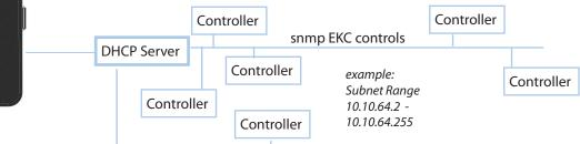
Check the box marked 'Channel SNMP'. SNMP is the protocol used to communicate with the EKC snmp controllers. Enter an address range for the AK-SC255 to scan in order to detect the EKC devices. For example, settings as IP address range (10.10.64.2 - 10.10.64.255).
