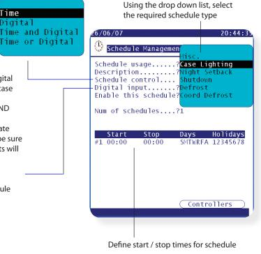
If using a digital point from a controller (import function), expect to see a time lag when the schedule gets activated after a change of switch input. This is due to network and system bus loads & speeds.
