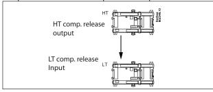
When a compressor is running in the high-pressure circuit, the controller will also pull the relay with the release signal into the low-pressure circuit.
