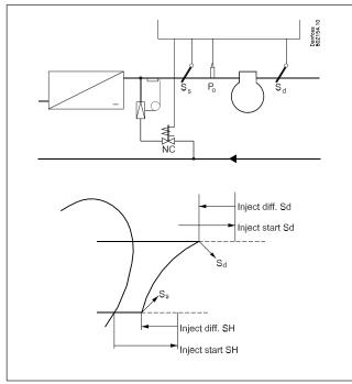
The high-pressure gas temperature can be kept down by means of liquid injection into the suction line.
