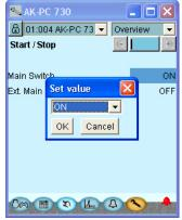
Press in the fileld against **Main switch**. Select **ON**. Press **OK**. The controller will now start controlling the compressors and the fans.
