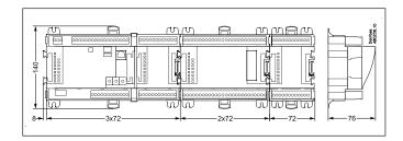
Example continued: Controller module + 1 extension module in 100-series = 224 + 72 = 296 mm.
