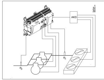
The controller's main function is to control compressors and condensers so that operation all the time takes place at the energyoptimum pressure conditions. Both suction pressure and condensing pressure are controlled by signals from pressure transmitters. Capacity control can be carried out by suction pressure P0, media temperature S4 or separate control pressure Pctrl (for cascade).
