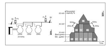
As the variable part of the speed controlled compressor is smaller than the following compressor steps the capacity curve will have some holes that can not be filled out by the variable capacity.
