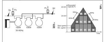
As the variable part of the speed controlled compressor is bigger than the following compressor steps, the capacity curve will be without holes.
