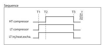
T1: The load on the low-pressure circuit requires compressor capacity.
