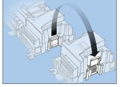
Remove the protective cap from the connection plug on the right-hand side of the basic module.
