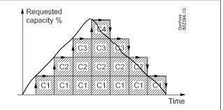
Cut-out of the last compressor stage:
