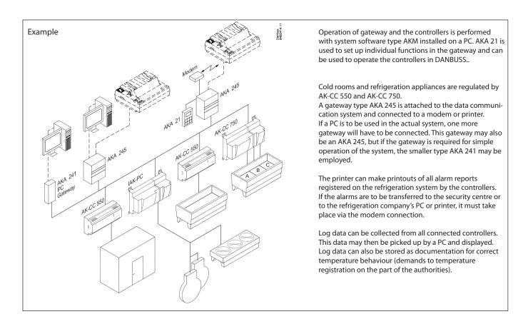
There are two data communication connections: • Lon RS 485, for controller types AK-CC and EKC
