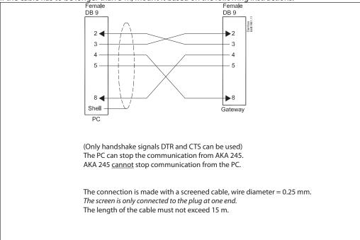
If there is a USB drive, but no serial port on the PC, connection can be made via a converter between the USB drive and the serial cable, e.g. type "Digi Edgeport/1".
