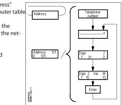
The actual telephone number for the selected line in the router table. The telephone number may consist of up to max. 30 significant digits composed of figures and modem codes. All telephone numbers must be terminated with 'x' (see below).
