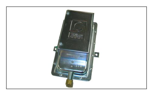
The CAFS-1 is a duct-mounted air flow switch that provides a signal to your Danfoss environment control system to ensure that fans are properly functioning. The CAFS-1 is typically set to alarm in the open position, indicating a cessation of air flow. The switch can also be set to detect a pressure differential across an air filter, indicating the need to change the filter.
