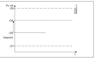
If you need to raise the condensing temperature for, say, heat recovery, an offset value (r34) has to be set. The DI5 function must be defined to 1.
