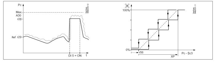
As "2", but an increasing deviation from the reference must be accepted as the controller uses the difference between the actual condenser temperature and the actual outdoor temperature for indicating the number of fans that has to be cut in. (The first "r56-degrees" are left out, as there must be a possibility of cooling via the condenser).
