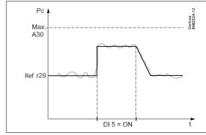
The reference at any time, on the basis of which the controller regulates, can be seen in "r29".
