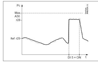
The reference follows the outdoor temperature Sc3. If the outdoor temperature drops one degree the reference will also drop one degree. The reference is adjusted according to the compressor capacity with max. Xp value.
