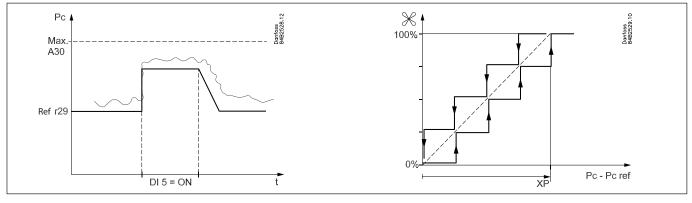
As "1", but an increasing deviation from the reference must be accepted as the controller uses the difference between the actual condenser temperature and the set reference for indicating the number of fans that has to be cut in. The number of fan steps is divided up based on the Xp value. Recommended setting for Xp is the  $\Delta T$  of the condenser, typically 10 to 15 K.
