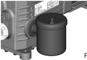
Mechanical oil level regulator at the "O" connection
