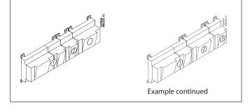
The modules are attached to one another and kept together by a connection which at the same time transmits the supply voltage and the internal data communication to the next module.
