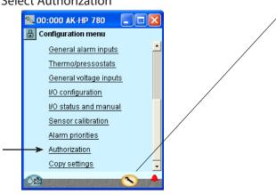
When the controller is supplied it has been set with standard authorization for different user interfaces. This setting should be changed and adapted to the plant. The changes can be made now or later.
