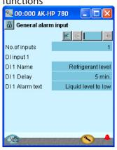
In our example we select one alarm function for monitoring the liquid level in the receiver. We have subsequently selected a name for the alarm function and for the alarm text.
