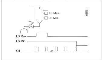
The system can be controlled by a signal from a high level switch or it can be controlled by a signal from both a high and a low level switch.
