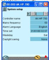
All system settings can be changed by pressing in the blue field with the setting and then indicating the value of the required setting.
