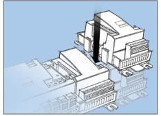
In our example two extension modules are to be fitted to the basic module. We have chosen to fit the module with relays directly on the basic module and then the module with input signals. The sequence is thus:
