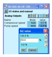
6. Put the control of the output voltage back to automatic
