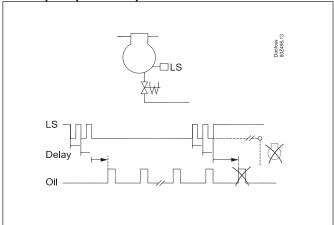
A compressor that is shut down does not receive any oil. When the compressor is in operation, a signal from the compressors oil-level switch is expected. When the signal is given, the following process is carried out:
