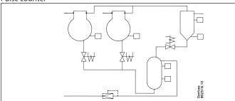
Here, the controller uses a pulse count to determine the pressure build-up in the receiver.
