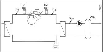
P0 is used as a safety function for low suction pressure and will ensure disconnection of compressor capacity
