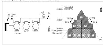
As the variable part of the speed controlled compressor is smaller than the following compressor steps the capacity curve will have some holes that can not be filled out by the variable capacity.
