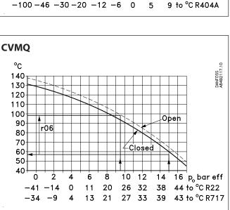
The two curves are shown with the valve's spring setting equal-ling the factory setting. If the spring setting is changed to a higher pressure, the curve will be displaced correspondingly to a higher temperature.
