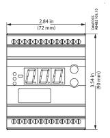
Mounting: DIN rail Enclosure: IP 20 Weight: 0.66 lbs (300 g)
