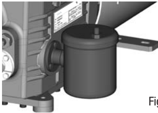
Mechanical oil level regulator at the "O" connection
