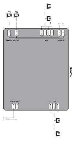
${}^*\!NOTE: connection\ has\ to\ be\ made\ on\ the\ first\ and\ last\ local\ network\ units.\ Make\ the\ connection\ as\ close\ as\ possible\ to\ the\ connector$
